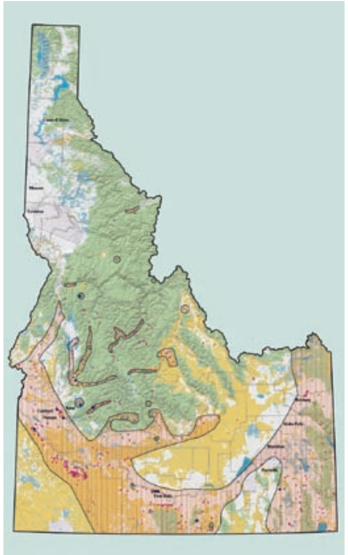
Geothermal resource map of Idaho, showing areas in pink with potential for direct-use applications (mostly lower half of State).
